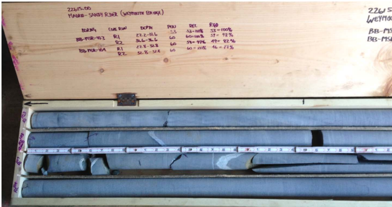
Photo 3: Core box containing rock core from test borings BB-MSR-103 and BB-MSR-104- left side of core box (top portion of cores). From top to bottom 1) BB-MSR-103, R-1; 2) BB-MSR-103, R-2; 3) BB-MSR-104, R-1; 4) BB-MSR-104, R-2.
