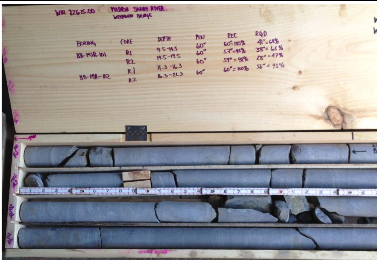
Photo 1: Core box containing rock core from test borings BB-MSR-101 and BB-MSR-102- left side of core box (top portion of cores).
