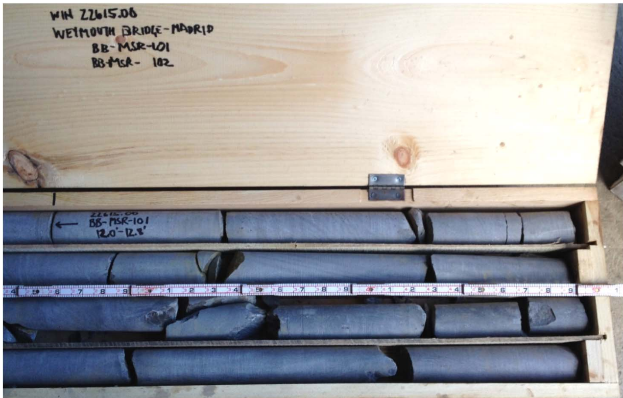
Photo 2: Core box containing rock core from test borings BB-MSR-101 and BB-MSR-102 – right side of core box (bottom portion of cores).
