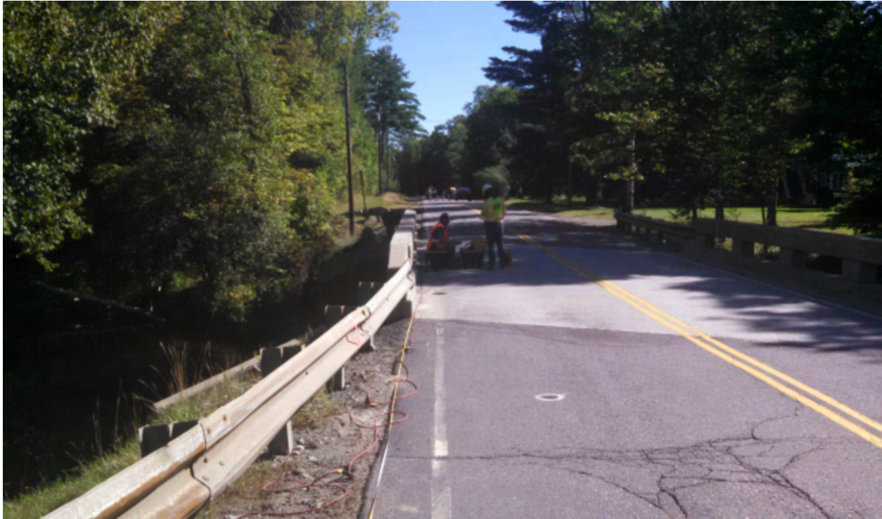
Photograph of Line 2 across the Weymouth Bridge, looking east. Geophones are planted in the gravel shoulders on either side of the bridge. The seismograph and operator are located in the center of the bridge.
